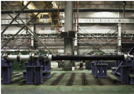
Carbon Fibre Shaft combined with LAMIDISC® coupling.
