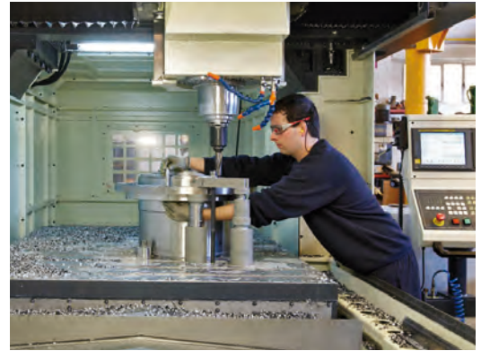
Machining of barrel coupling's hub.
