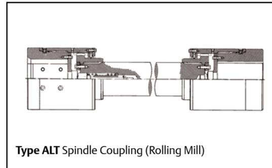
Type ALT Spindle Coupling (Rolling Mill)
