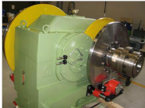
Jaure gear coupling with brake for hoisting
