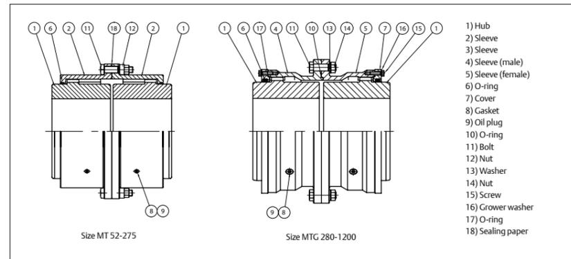
Fig n°1. Coupling components
