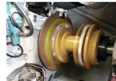
Torque monitoring on wind turbines.
