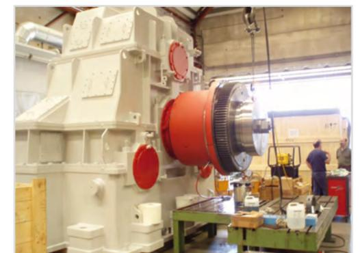
Jaure MTGX-HD-TI-1000 on wind test bench
