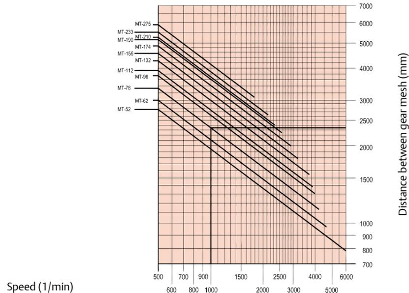
Ex.: MTD-78 with an intermediate shaft of 2350 mm can rotate at a speed maximum 1000rpm
