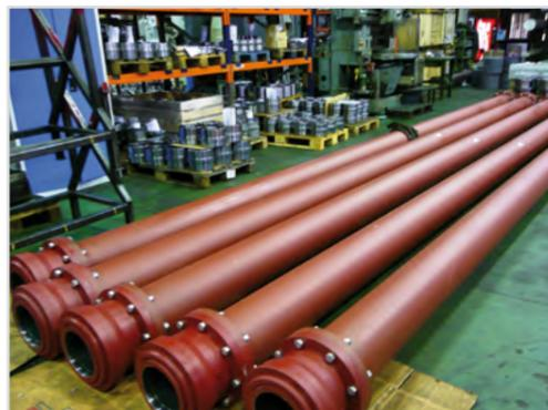
Jaure gear coupling for underwater operation
