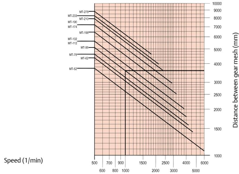
Ex.: MTX-98 with a spacer of 3575 mm can rotate at a speed maximum 1000 rpm
