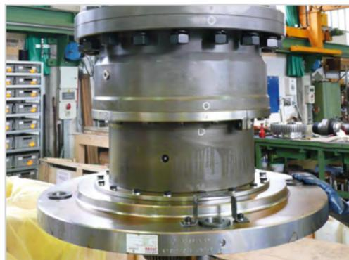
Shear pin type gear coupling
