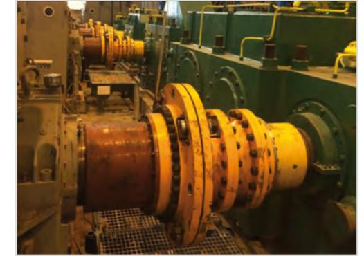
Shear pin gear couplings in steel mill
