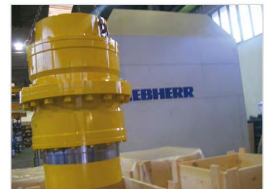
Packing of MTG-HD gear coupling
