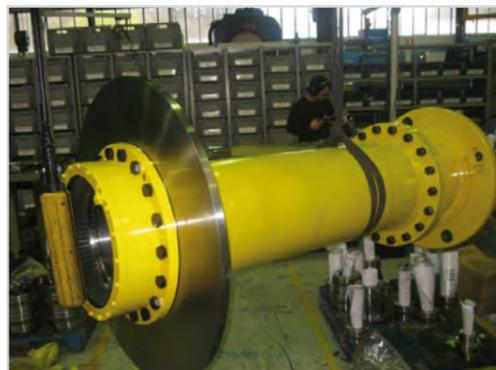
Gear coupling with brake
