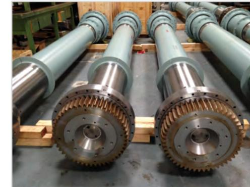
Case carburized gear spindles
