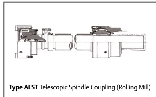
Type ALST Telescopic Spindle Coupling (Rolling Mill)
