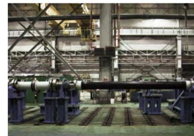
Carbon Fibre Shaft combined with LAMIDISC® coupling.
