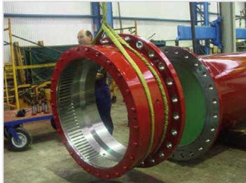
Intermediate gear coupling for HRM
