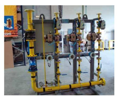
Operation is automatic. When the program reaches the pilot and lance modes, the natural gas cut-off valve will close and the nitrogen lines will open. The same alarms will be programmed for nitrogen (minimum pressure, maximum pressure, etc.) as those currently existing for the oxygen and natural gas lines.
