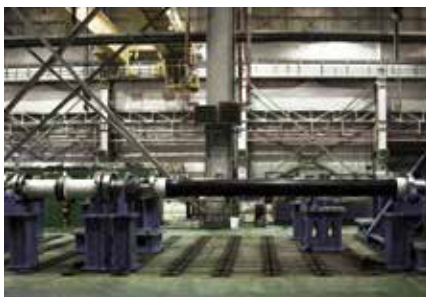
Carbon Fibre Shaft combined with LAMIDISC® coupling.
